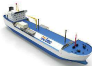
Figure 3. A 8000 m 3 LNG bunkering vessel: engineering development for a Singapore client to supply LNG to storage units and vessels.
