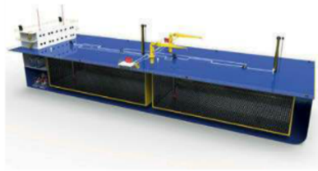
Figure 1. A 26 000 m 3 floating storage unit (FSU): turnkey design and build proposal for an Indonesian customer.
