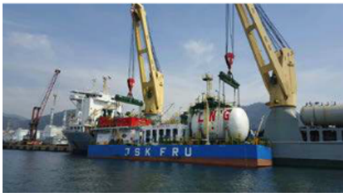
Figure 4. Bali Benoa 50 million ft 3 /d LNG FRU: GAS Entec delivered the world’s first small scale FRU for the 200 MW Bali Benoa gas-fired power plant.
