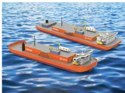
Figure 1. AG&P ultra-shallow draft LNG carrier in 2000 – 8000 m 3 carrying capacities offering a hull design optimised for shallow water LNG shuttle services to remote LNG receiving points.
