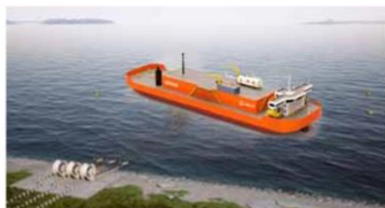
Figure 2. AG&P's ultra-shallow draft LNG carrier fitted with Trelleborg's Cryoline floating cryogenic transfer hoses, allowing for the safe and capital-efficient transfer of LNG in remote regions.
